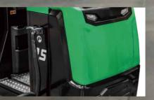
**Charging System:** It features a side charging design, with battery pack that can be lifted and removed from the side, making it convenient and quick.
